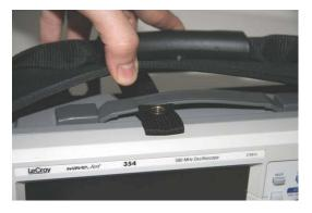
3. After threading the strap, slide it through the top case slot and fasten the snap.
